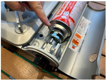
⑤ Place the cylinder in place, aligning it with the recessed cut.
